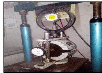
Figure 10 Marshall test of a DBM sample in progress.
