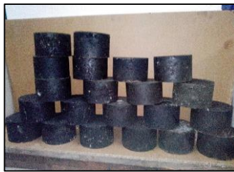
Figure 9 A view of DBM samples before Marshall testing.
