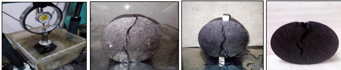
Figure 11 Loading of a specimen during ITS test and different views of specimens after ITS test.
