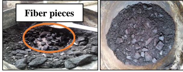
Figure 7 Addition of bitumen and fiber followed by thorough mixing.
