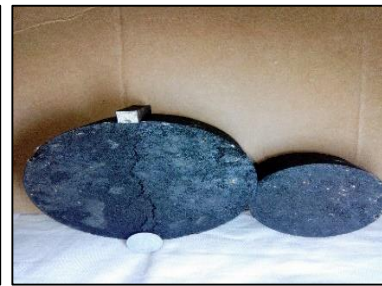
Figure 14 View of cracks in DBM sample after failure.
