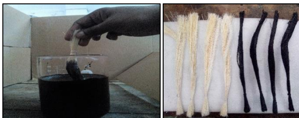
Figure 4 Coating of emulsion on fiber.
