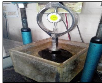
Figure 13 Moisture susceptibility test in progress.
