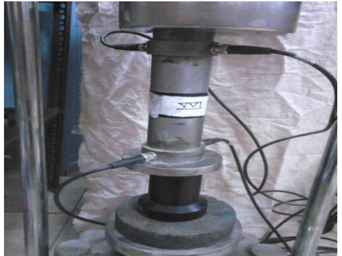
Fig. 4 Coal sample placed in between platens to pass sonic wave through it.
