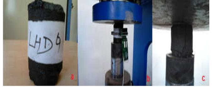
Fig. 3 (a) Coal core sample for testing (b) Sample placed between platen (c) Fracture profiles of sample after application of load
