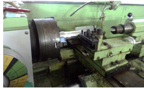
Fig.1 Photograph of experimental setup for turning of Inconel 825.
