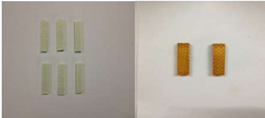
Figure 1. Glass/fibre composite before post curing and after post curing
