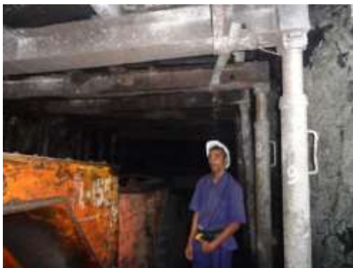
Fig 3: Remote LHD used in a typical mine (Blasting typical Gallery method)
