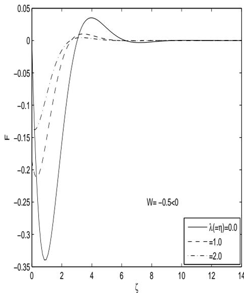
Figure 3: Variation of  $F$  with  $\lambda(=\eta)$  when  $W = -0.5$ .
