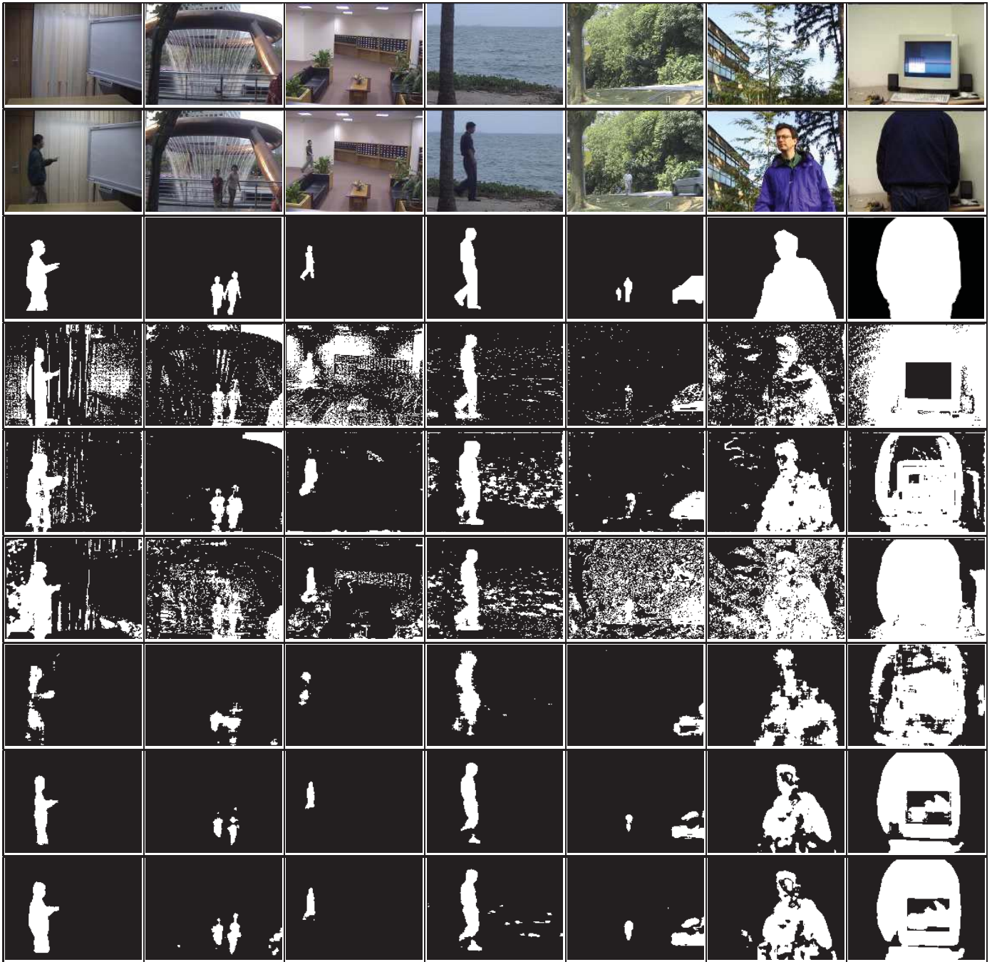
Fig. 5. Left to right: Curtain, Fountain, Lobby, Water Surface, Campus, Waving trees, Camouflage. Top to bottom: Original Image, Test Image, Ground truth, Moving object detection for GMM, Covariance BS, Moment BS, LBP BS, STBS, TCMS
