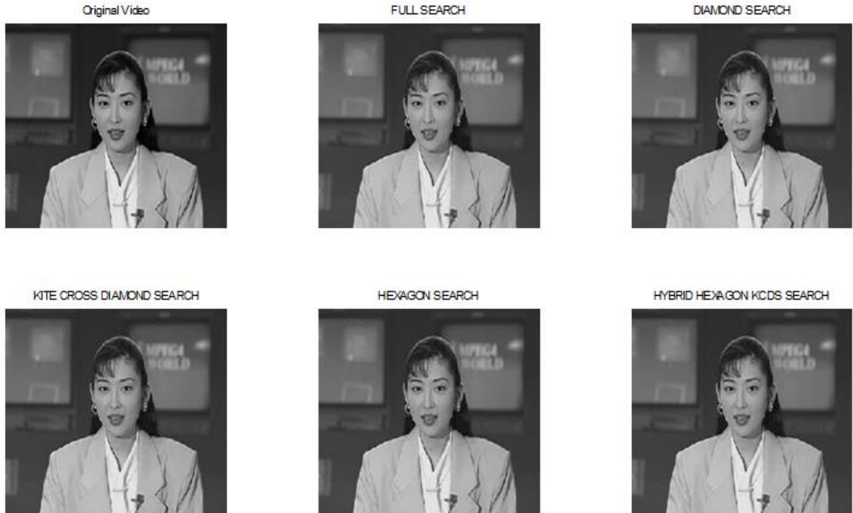
Fig.10. Frame 23 of the test video Akiyo_cif and its corresponding reconstructed frames using FS, DS, KCDS, HEXS and proposed HYBHKS algorithms.
