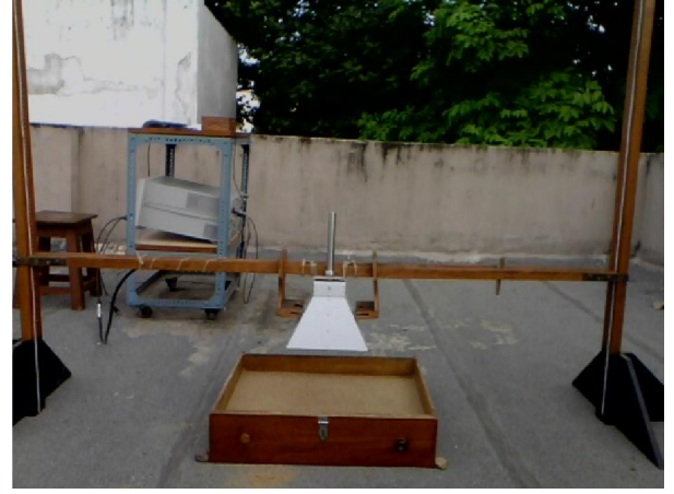
Figure 3: Picture of the GPR setup at roof top.
