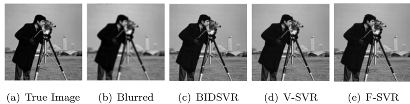
Figure 6: Restoration results of Cameraman image degraded with out-of-focus blur ( R = 5 ) by various schemes.
