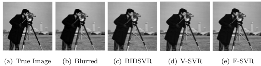
Figure 9: Restoration results of Cameraman image degraded with horizontal motion blur ( L = 5 ) by various schemes.
