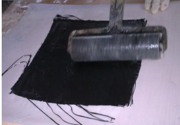
Figure 3 - Hand Lay Up method used for fabrication
