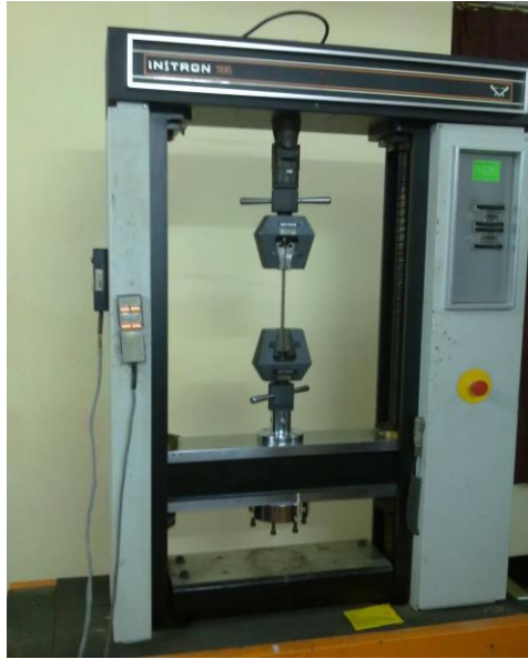
Figure 4: Tensile testing of CFRP plates using INSTRON 1195
