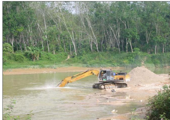
Fig 2 : Wet-Pit Channel Mining
