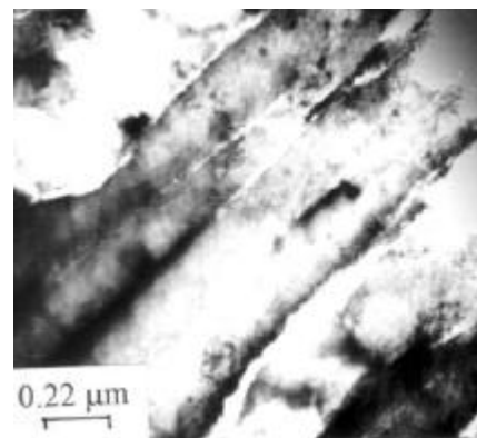
Fig. 5(b) - TEM of WQ steel showing precipitates within the laths. The white regions near lath boundaries are reported to be austenite.
