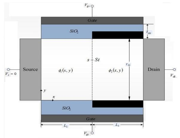
Fig.1. Cross sectional view of DG s-Si MOSFET
