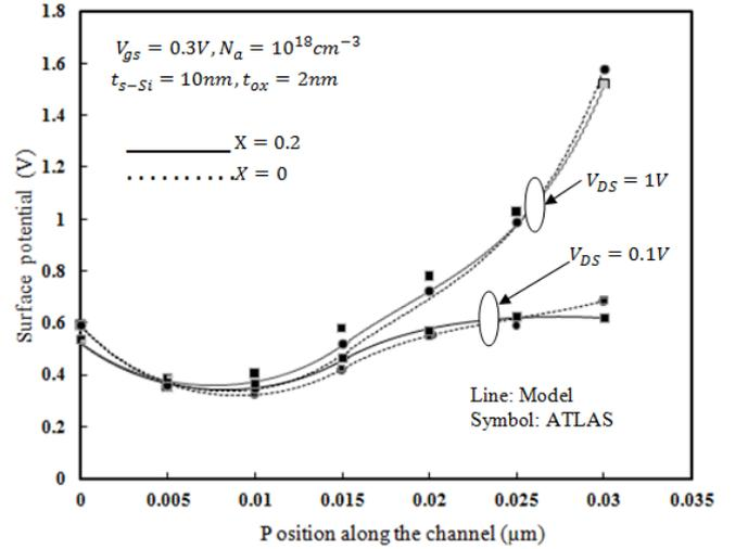
Fig. 5. Surface Potential along the channel length for different drain voltage and mole fraction variation
