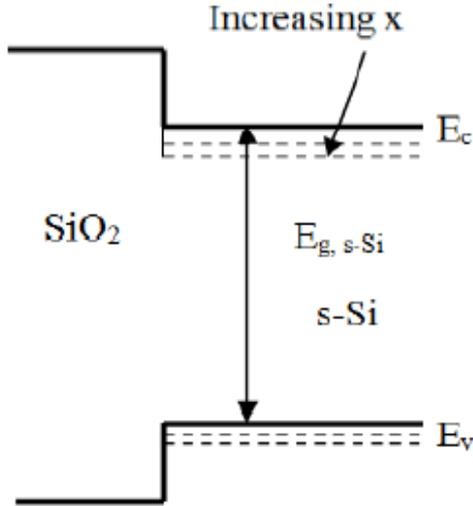
Fig. 2. Modified Silicon Band Structure due to strain
