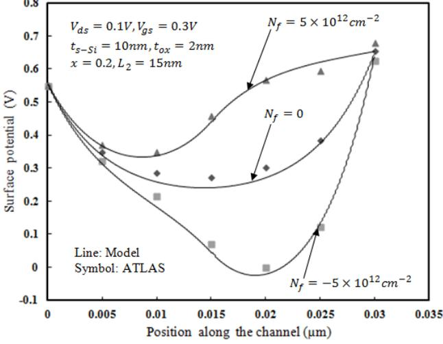
Fig. 3. The surface potential for charge variations (in magnitude and polarity)
