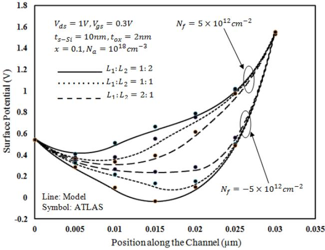
Fig. 4. The surface potential profile along the channel length for different length ratio ( $L_1:L_2$ ) of undamaged and damaged region
