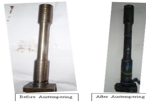
Fig. 2: Dog Bone Shaped Ductile Iron Before and After Austempering.
