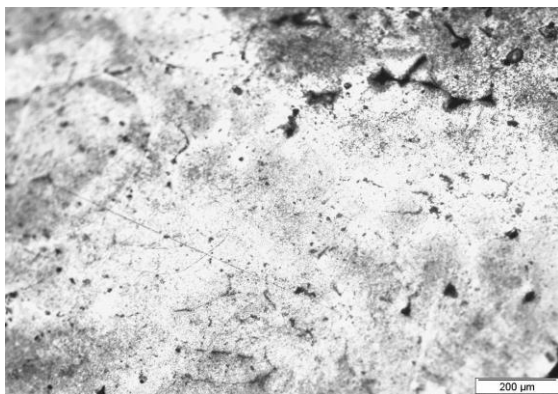
Fig. 5: The Microstructure of Al-1wt%Mg Alloy.
