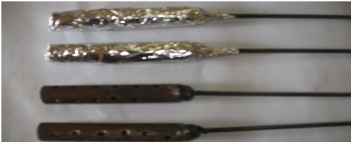
Fig. 2: Photograph of Capsule Welded to Plunger Rod.
