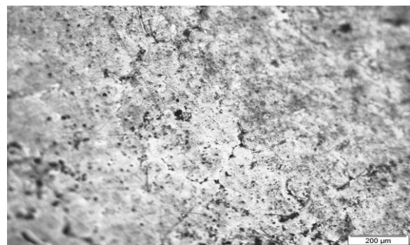
Fig. 8: The Microstructure of Al-7 wt%Mg Alloy.
