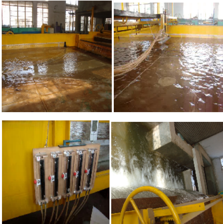
Fig2.(a-d),clockwise starting top left: (a)U/S rectangular notch entrance bell mouth section,,(b)Series of pitot static tube fitted to stand with transparent pipes & point gauge,(c) Set of Piezometers fitted to wooden board to record pressure with spirit level, digital clock etc.&(d)D/S tail gate and volumetric tank
