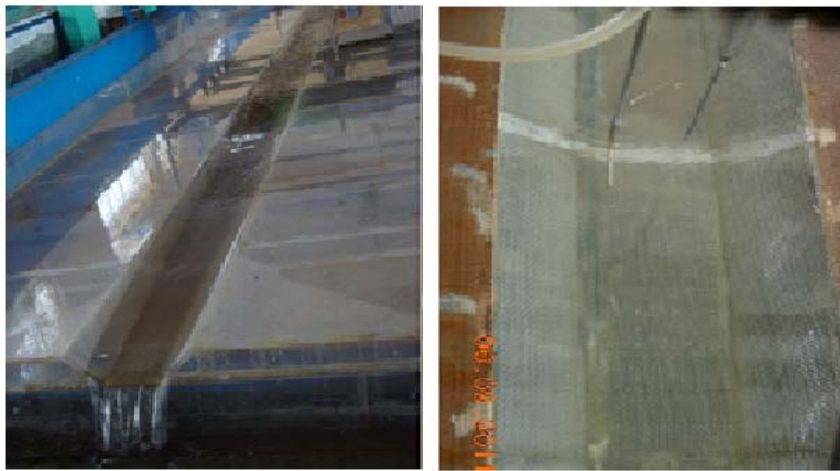
Fig. 2. Photographs of in-bank Flow for Determination of Manning's n of Perspex sheet and Wire-mesh
