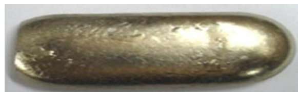
Fig. 1: Prepared Sample of \text{Ni}_{50}\text{Mn}_{37.5}\text{Sn}_{12.5} Heusler FSMA.
