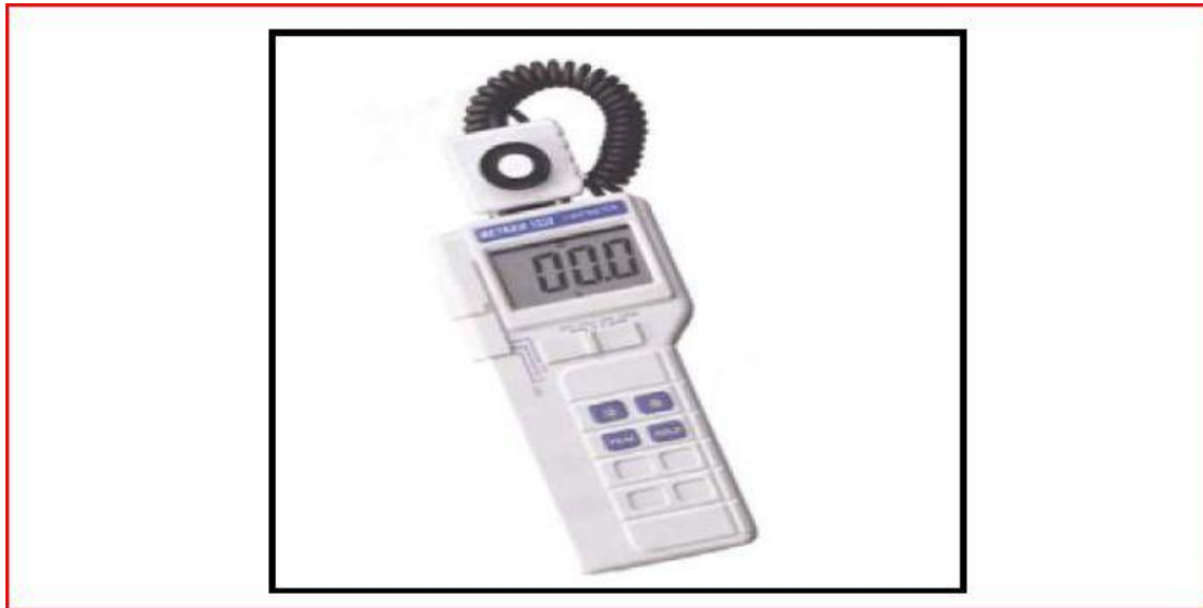
Fig 1 . Digital Luxmeter (MetraVi, 2011) for measuring illuminance
