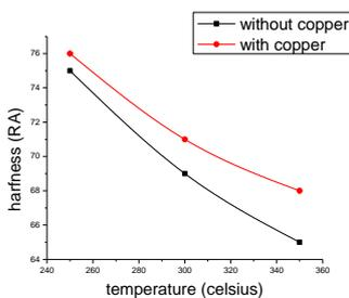
**Figure 4. Variation of hardness with respect to the austempering temperature for 30 min**
