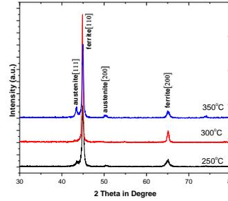
**Figure 10. XRD pattern of unalloyed ductile iron austempered for 60 min.**
