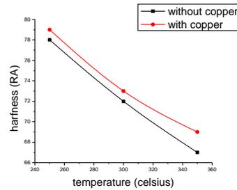
**Figure 7. Variation of hardness with respect to the austempering temperature for 120 min.**
