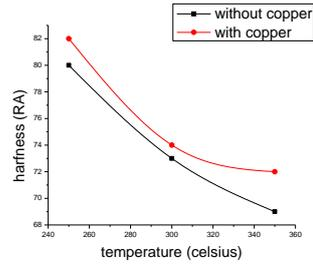
**Figure 5. Variation of hardness with respect to the austempering temperature for 60 min.**
