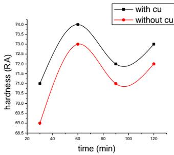
**Figure 2. Variation of hardness with respect to the austempering time at temperature 300°C**
