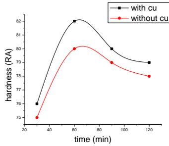
**Figure 1. Variation of hardness with respect to the austempering time at temperature 250°C**
