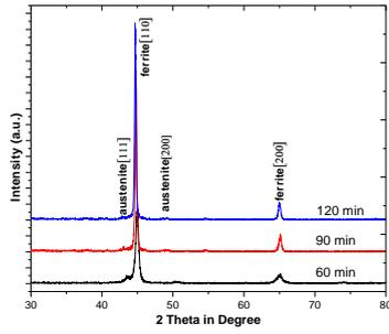
**Figure 8. XRD pattern of unalloyed ductile iron austempered at 250°C.**
