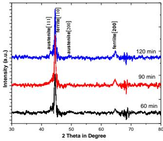
**Figure 9. XRD pattern of Cu alloyed ductile iron austempered at 250°C.**
