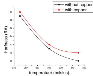
**Figure 6. Variation of hardness with respect to the austempering temperature for 90 min**
