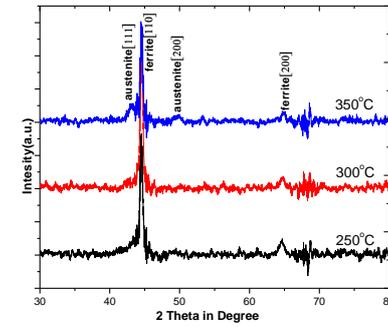
**Figure 11. XRD pattern of Cu alloyed ductile iron austempered for 60 min.**
