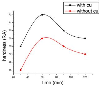
**Figure 3. Variation of hardness with respect to the austempering time at temperature 350°C**
