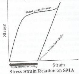
The potential for use of SMAs in engineering structures is limited by the range of temperatures within which phase change may take place and the rapidity with which these changes occur and most important factor is of higher cost. Many experiments exist based on the principle of using shape memory alloy element as a thermal actuator which converts thermal energy into mechanical work. Recent interest in the development is
