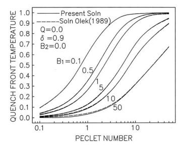
Figure 7. Quench front temperature variation with Biot and Peclet number for the tube with  $\delta = 0.9$
