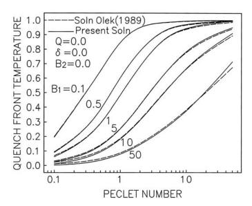
Figure 8. Quench front temperature variation with Biot and Peclet number for the rod  $(\delta = 0)$
