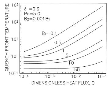
Figure 4. Quench front temperature for various heat flux and Biot numbers
