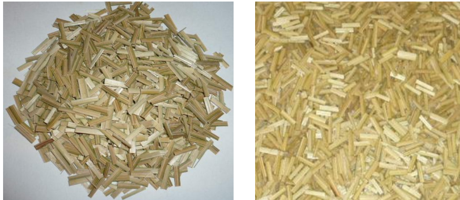
Figure 1 Short bamboo fiber and bamboo based composite
