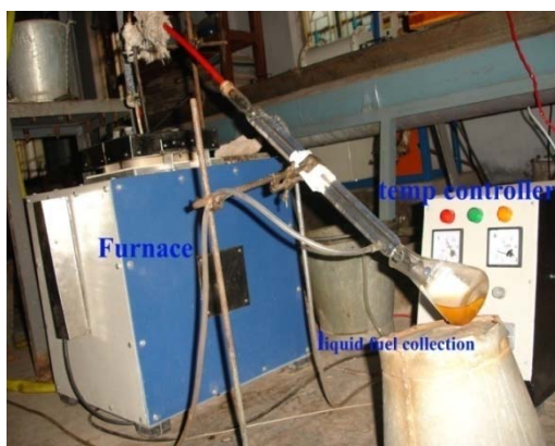
Fig.1(a) SBR Experimental setup Fig.1(b) Liquid fuels of PP with various catalysts to feed ratios.
