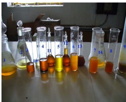
Fig.1(a) SBR Experimental setup Fig.1(b) Liquid fuels of PP with various catalysts to feed ratios.
