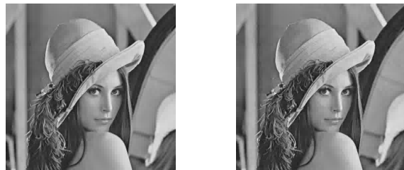
Fig. 4. The reconstructed images of Lena using HVS based DTT-SPIHT at a bit-rate of 0.25 bpp (a) HVS on (PSNR=31.5) (b) HVS off (PSNR=31.6).
