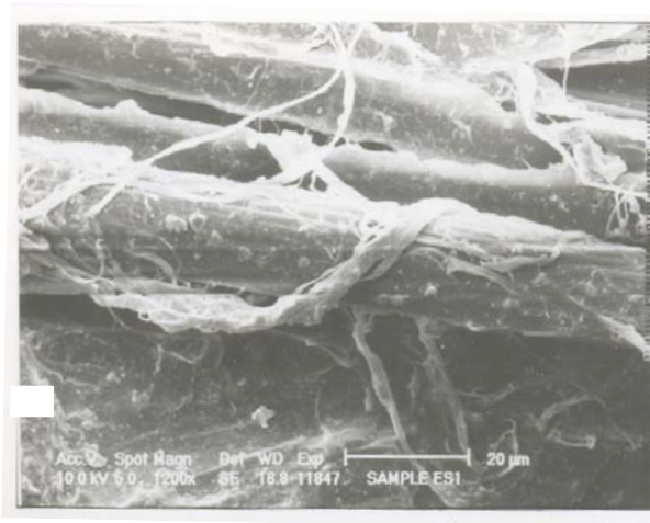
Fig.2: SEM micrograph showing fibrillar morphology on the delaminated surfaces.
