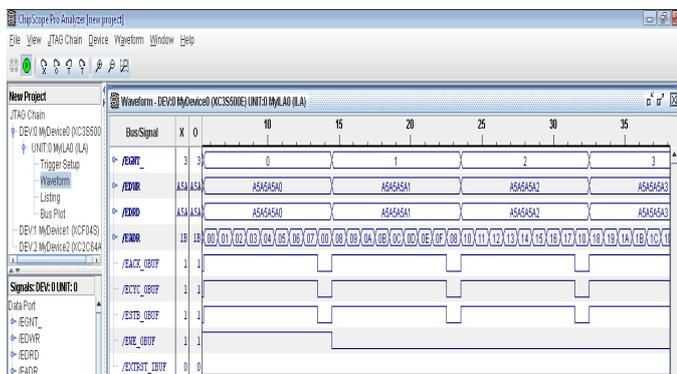
Fig. 6: Board Level Verification Results of Shared bus Architecture
