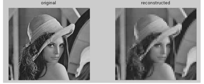
Fig.1. Original and Reconstructed lena image after taking only DC coefficients of each block.
