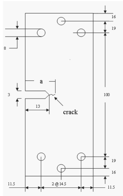
Fig. 1. Geometry of the SENT specimen (dimensions in mm)
