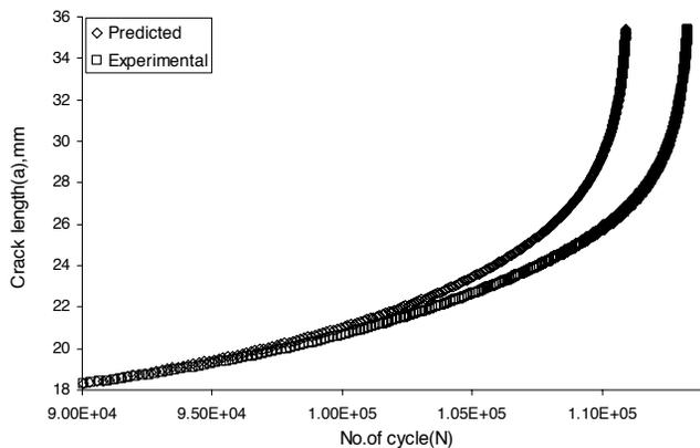
Fig. 10. Comparison of predicted (ANN) and experimentally obtained crack length with number of cycle ( $N$ ) for load ratio 0.5 (2024 T3 alloy)
