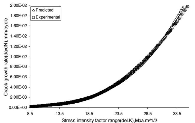
Fig. 8. Comparison of predicted (ANN) and experimental crack growth rate with stress intensity range ( $\Delta K$ ) for load ratio 0.5 (2024 T3 alloy)
