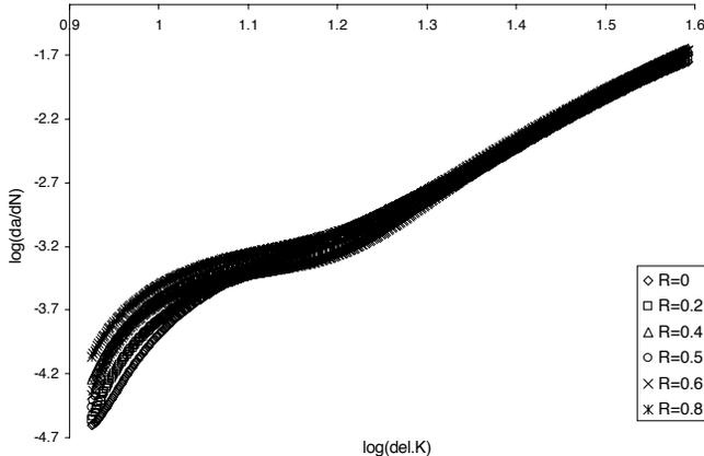
Fig. 5. Comparison of  $da/dN \sim \Delta K$  curves for different load ratios (7020-T7 alloy)
