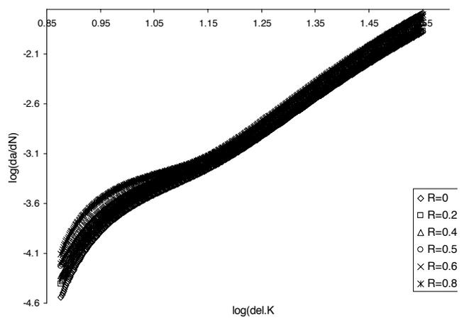
Fig. 6. Comparison of  $da/dN \sim \Delta K$  curves for different load ratios (2024-T3 alloy)
