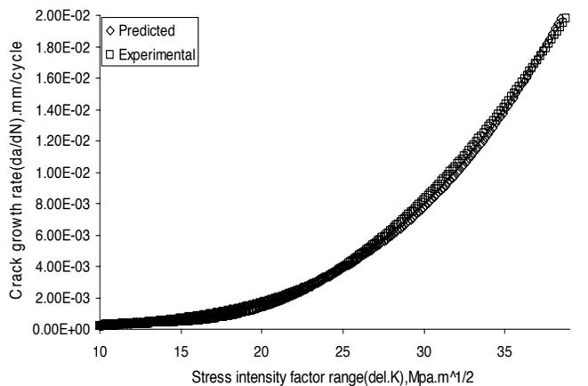
Figure 7. Comparison of predicted (ANN) and experimental crack growth rate with stress intensity range ( $\Delta K$ ) for load ratio 0.5 (7020 T7 alloy)
