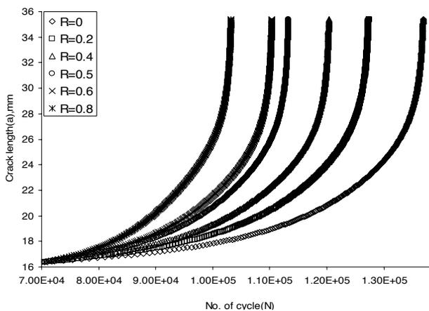
Fig. 4. Comparison of  $a \sim N$  curves for different load ratios (2024 T3 alloy)
