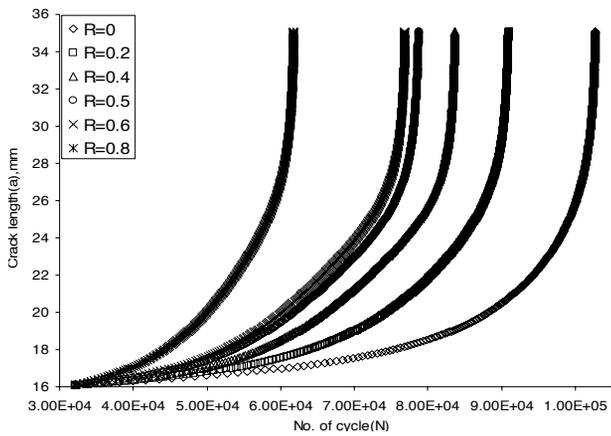
Fig. 3. Comparison of  $a \sim N$  curves for different load ratios (7020 T7 alloy)
