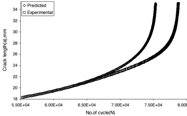
Fig. 9. Comparison predicted (ANN) and experimentally obtained crack length with number of cycle ( $N$ ) for load ratio 0.5 (7020 T7 alloy)
