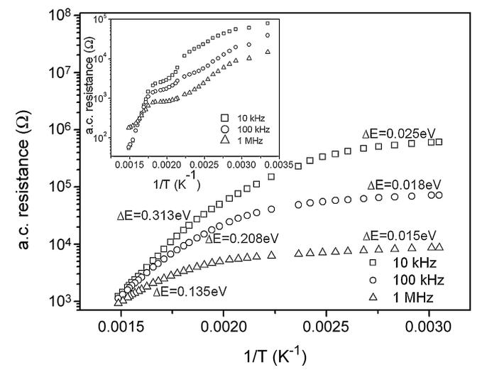
Fig. 9. ac resistance vs. inverse absolute temperature plots for SPS675 sample at different frequencies and (inset CS sample).
