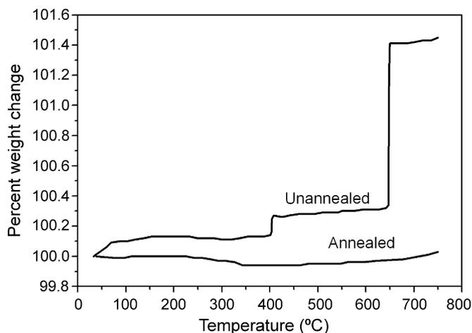
Fig. 3. TGA curves of as-sintered and annealed SPS samples.
