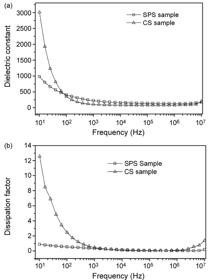
Fig. 6. Variation of (a) dielectric constant and (b) dissipation factor with frequency (at room temperature) for CS and SPS675 samples.
