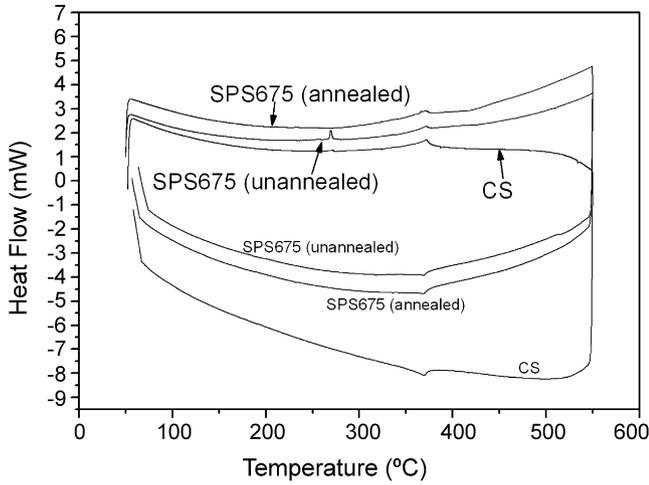
Fig. 4. Differential scanning calorimetry traces of an annealed and an unannealed SPS sample and a CS sample.
