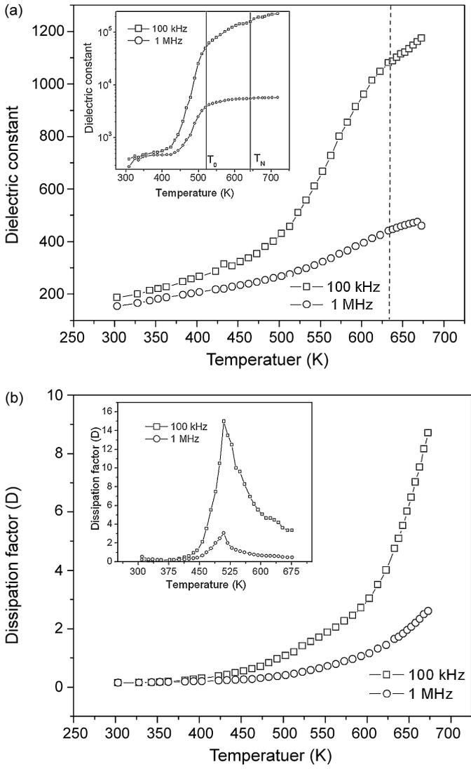
Fig. 7. (a) Dielectric permittivity and (b) dissipation factor vs. temperature for the SPS sample at 100 kHz and 1 MHz frequency (inset CS sample).
