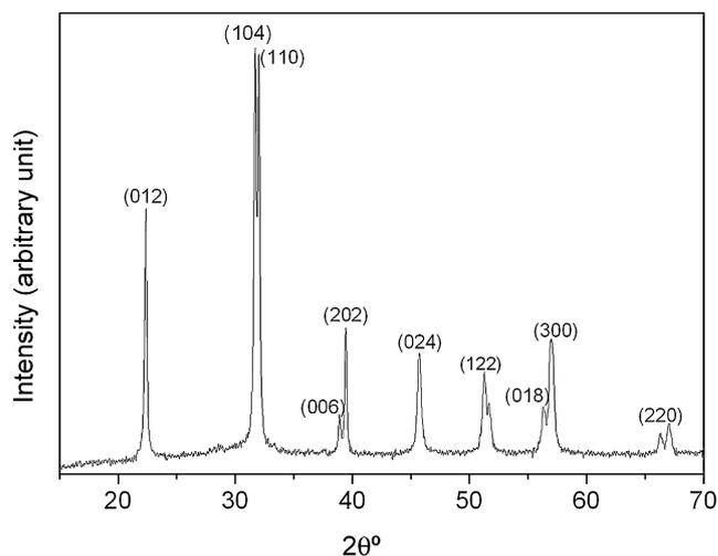
Fig. 1. X-ray diffraction pattern of calcined  $\text{BiFeO}_3$  powder.
