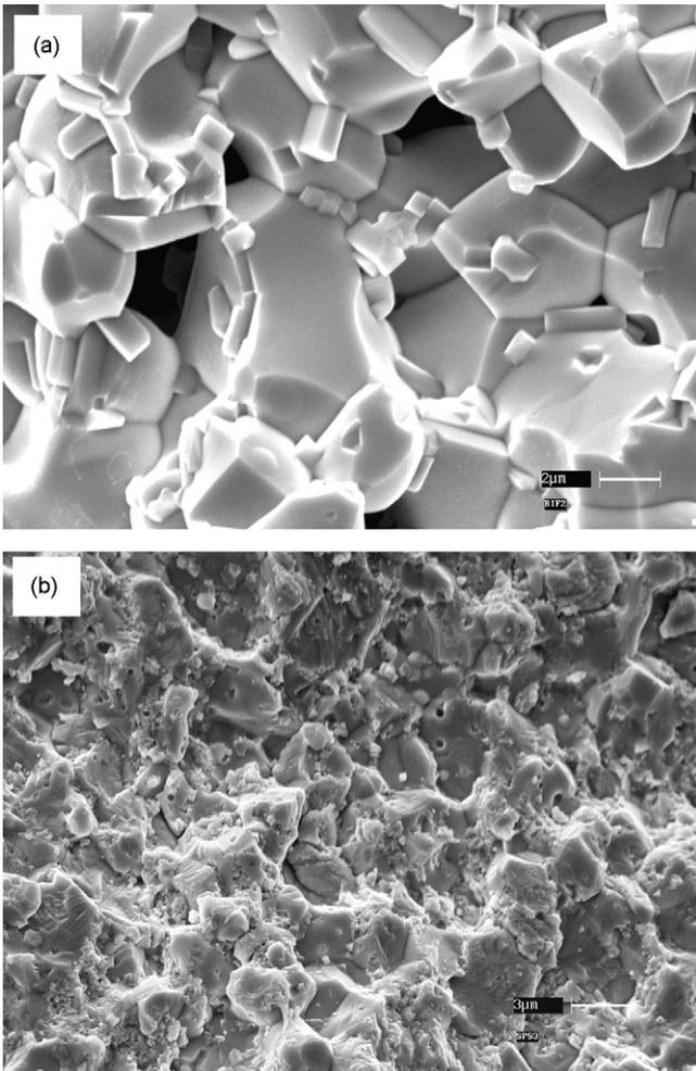
Fig. 5. SEM micrographs of fracture surfaces of (a) CS and (b) SPS675.
