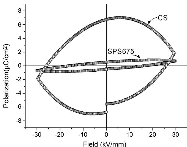
Fig. 10.  $P$ - $E$  hysteresis loops of CS and SPS675 samples.
