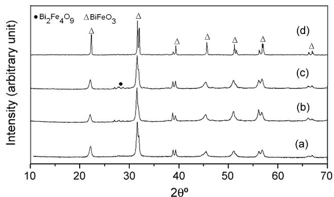
Fig. 2. X-ray diffraction patterns of ground SPS pellets after sintering at different temperatures (a)  $675^\circ\text{C}$ , (b)  $700^\circ\text{C}$ , (c)  $750^\circ\text{C}$  and (d) conventionally sintered (CS) pellet (and ground  $830^\circ\text{C}$ ).
