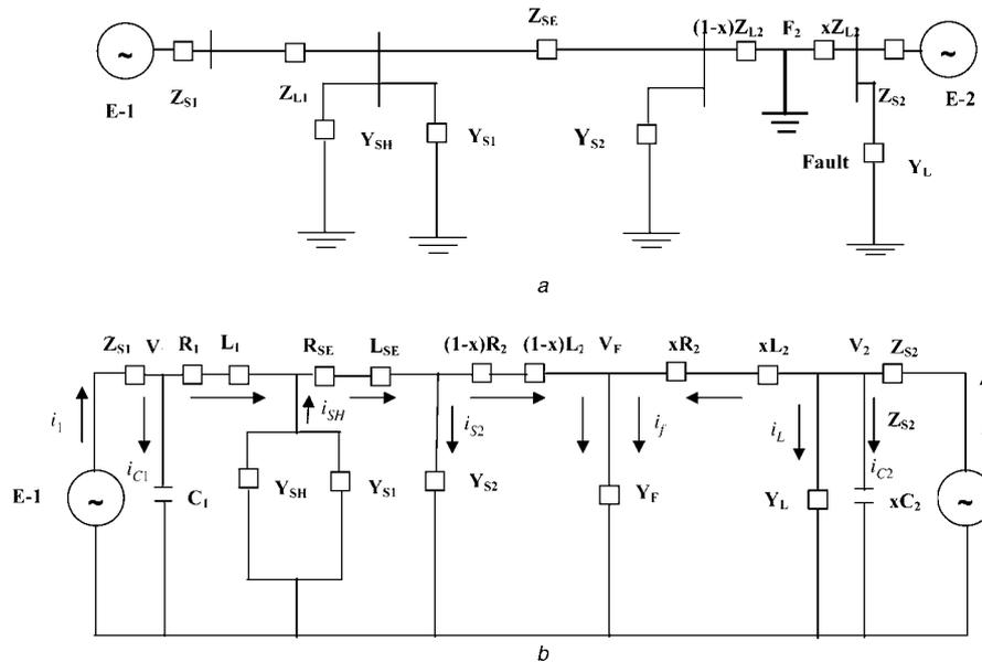
**Figure 6** UPFC-based line and equivalent model for fault at F2
