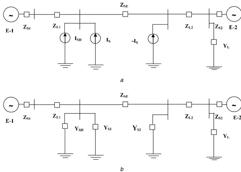
**Figure 4** Equivalent current injection and admittance model
