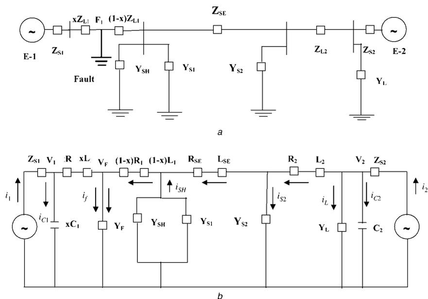
**Figure 5** UPFC-based line and equivalent model for fault at F1
