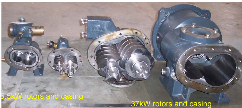
Figure 3: Photograph of 5.5 kW and 37 kW compressor rotors and their casings.
