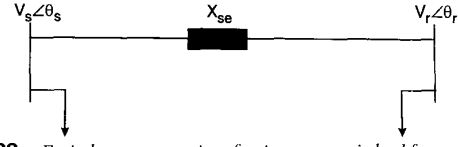
Fig. 28 Equivalent representation of series converter in load form
