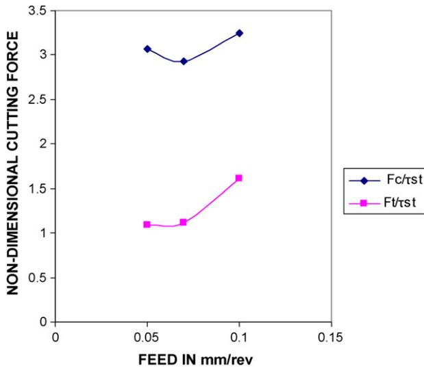
Fig. 8 – Variation of non-dimensional cutting force and thrust force with respect to time.
