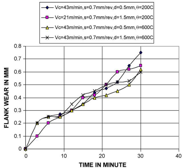
Fig. 5 – Variation of width of flank wear land with respect to time for third set of cutting variables.
