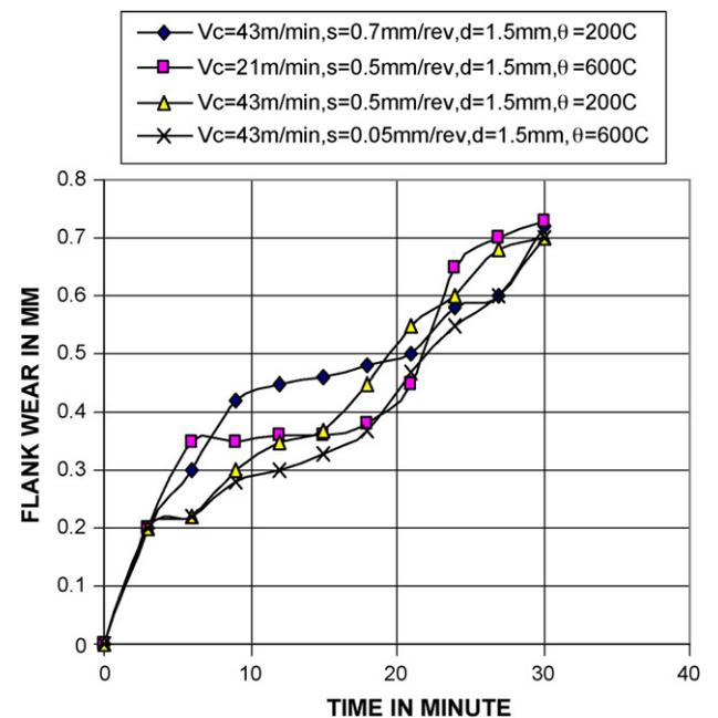
Fig. 6 – Variation of width of flank wear land with respect to time for fourth set of cutting variables.
