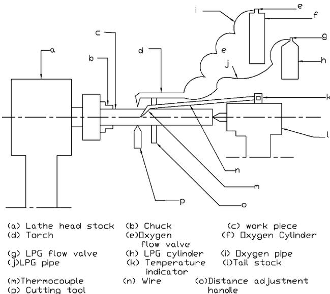
**Fig. 2 – Schematic diagram of experimental set-up.**
