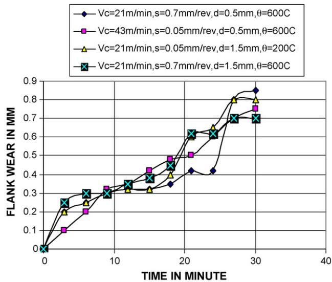
Fig. 4 – Variation of width of flank wear land with respect to time for second set of cutting variables.
