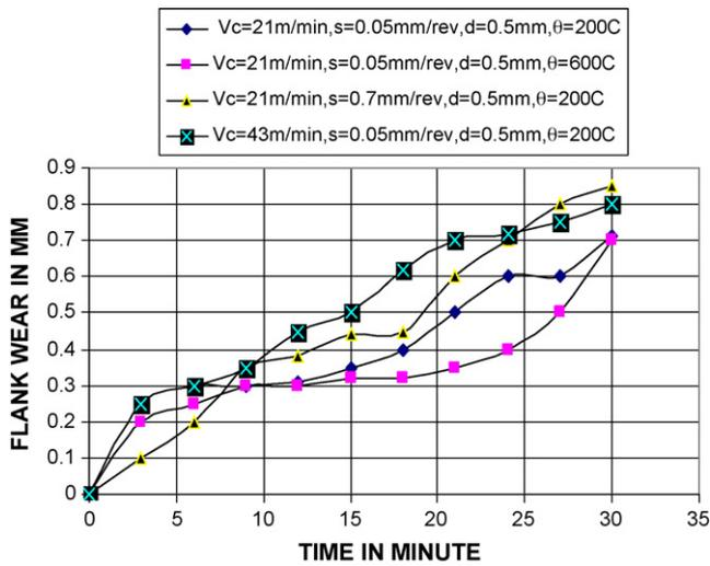
Fig. 3 – Variation of width of flank wear land with respect to time for first set of cutting variables.
