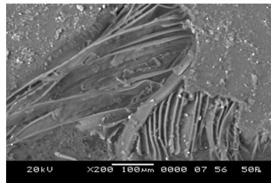
Figure 2 SEM Micrograph of composite eroded \alpha=90^{\circ}
