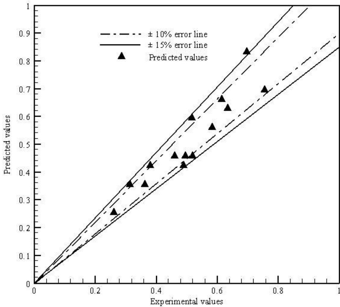
Fig. 7: Comparison between experimental values with predicted values of flank wear by 5-15-1 architecture in SOM
