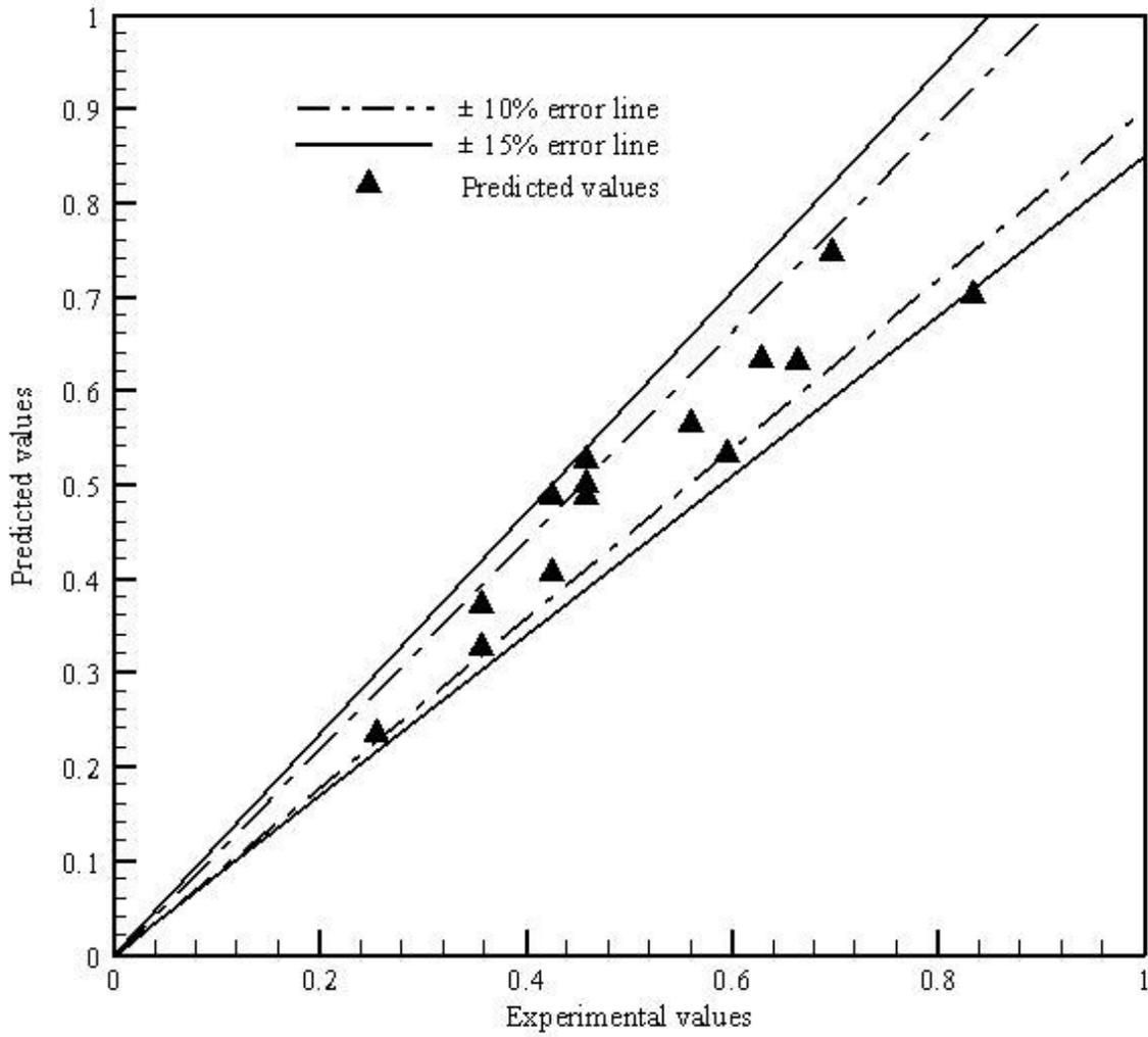
Fig. 3: Comparison between experimental values with predicted values of flank wear by 5-20-1 architecture fixed center selection in sample mode (for  $\alpha = 0.3$ ,  $\eta = 0.3$ ).
