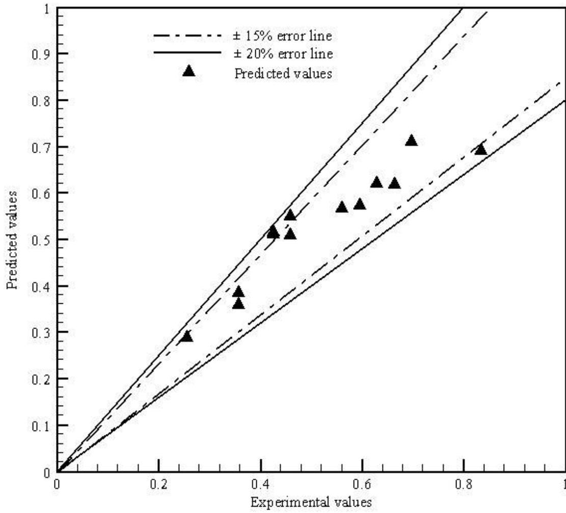
Fig. 5: Comparison between experimental values with predicted values of flank wear by 5-20-1 architecture fixed center selection in batch mode (for  $\alpha=0.4, \eta=0.7$ ).
