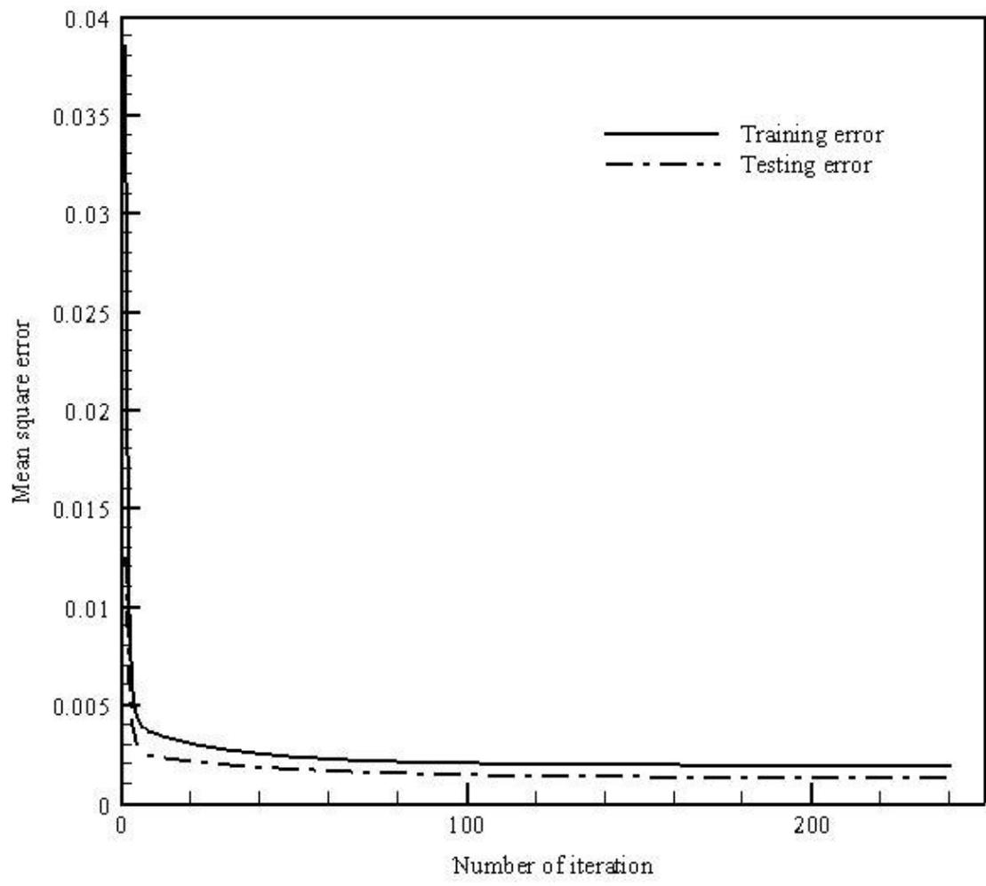
Fig.2: Variation of mean square error with number of iteration of 5-20-1 architecture fixed center selection in sample mode (for  $\alpha=0.3$ ,  $\eta=0.3$ ).
