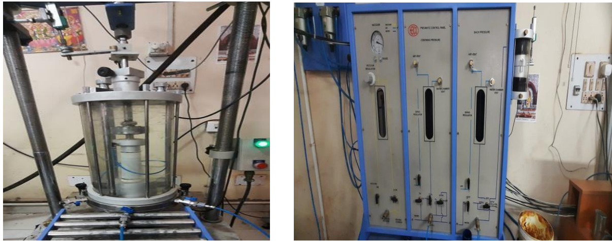
Figure 3: Triaxial Cell and Pneumatic Control Panel
