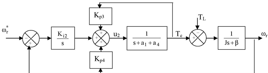
Fig. 2. Block diagram of the mechanical subsystem with SFC
