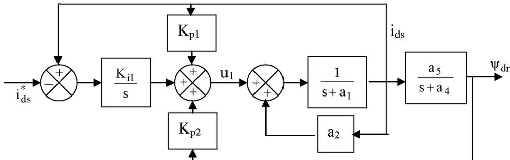
Fig. 1. Block diagram of the electrical subsystem with SFC
