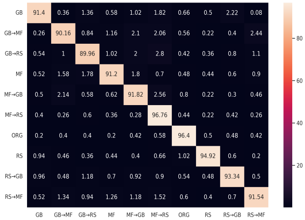
Fig. 5: Confusion matrix to identify operator chain detection (i.e. JPEG-series of manipulations-JPEG) with the proposed framework.
