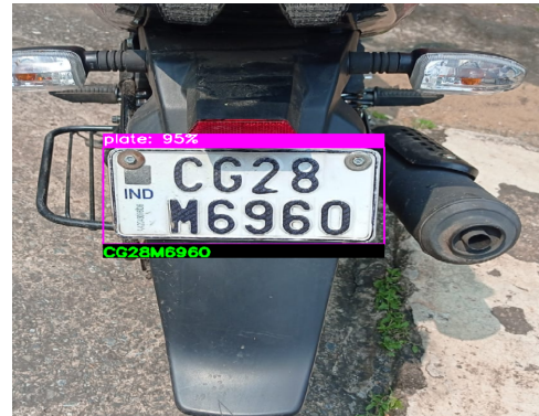
Fig. 7: Output after performing OCR
