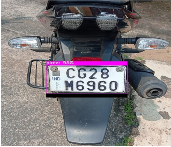
Fig. 4: Image after registration plate detection using YOLOv5 Model
