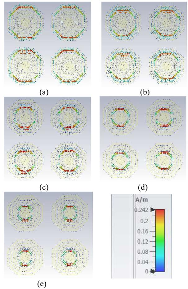
Fig. 8. Current distribution plots (a) 4.563 GHz, (b) 5.550 GHz, (c) 6.947 GHz, (d) 8.333 GHz, and (e) 10.402 GHz.
