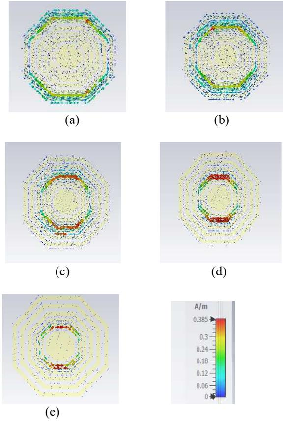
Fig. 5. Current distribution plots (a) 4.477 GHz, (b) 5.484 GHz, (c) 6.833 GHz, (d) 8.201 GHz, and (e) 9.816 GHz.
