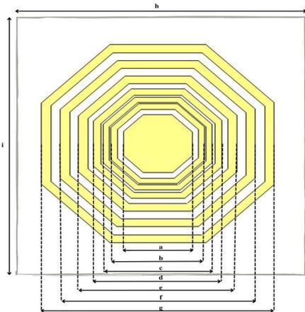
Fig. 3. The structure of orthogonal resonator based transponder.
