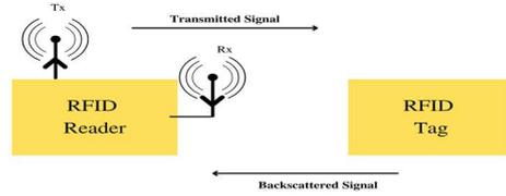
Fig. 2. RFID operation.
