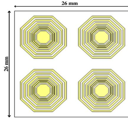
Fig. 6. Structure of octagonal unit array.
