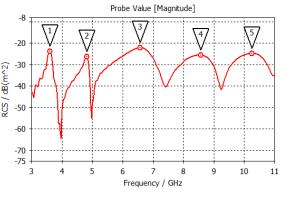
Fig. 6. RCS response curve of transponder 2.
