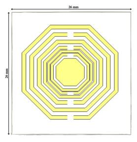
Fig. 5. Structure of transponder 2.
