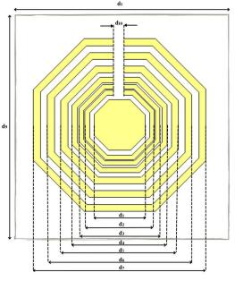
Fig. 2. Structure of transponder 1.
