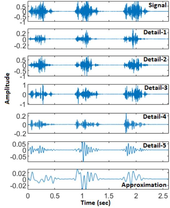
Fig. 4. Obtained detailed and approximation level signal using DWT decomposition
