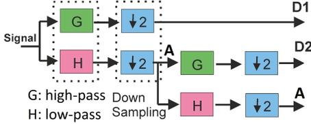
Fig. 3. Decomposition steps according to Mallat's subband coding algorithm
