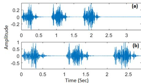
Fig. 2. Pre-processing of the signal (a) original signal, (b) resized and normalized signal
