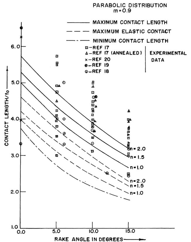
Fig. 5. The variation of maximum total contact length and maximum elastic contact length per unit undeformed chip thickness and exponents of distribution of normal stress.
