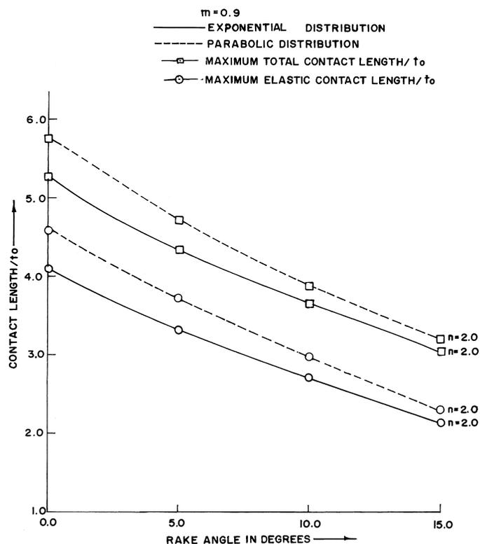
Fig. 6 indicates that both total contact length and the elastic contact length per unit undeformed chip thickness are greater for the case of the power-law distribution of normal stress than that of the exponential distribution in the elastic zone.
