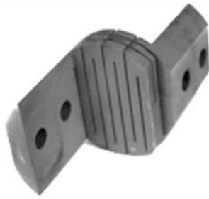
Figure 1. Magnetoresistive heat switch [9,10].
