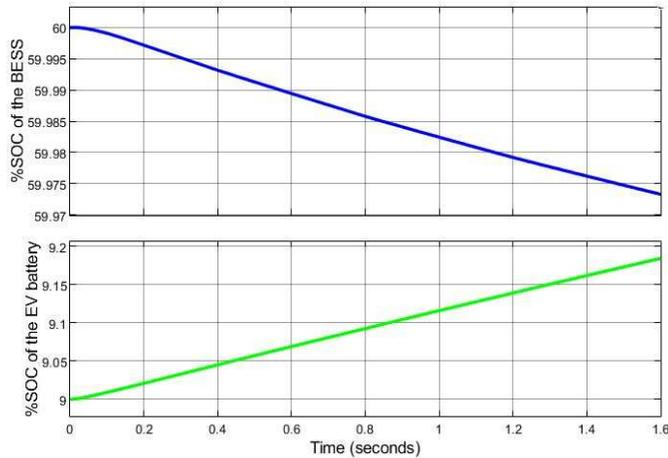
Fig. 15. BESS supplying energy to DC bus and Charging of EV battery
