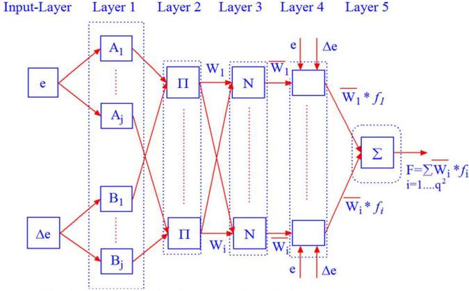
Fig. 2. Five-layer adaptive neuro-fuzzy inference system structure
