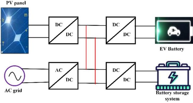
Fig. 1. Representation of EV charging station
