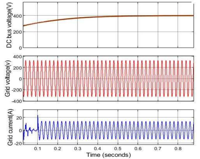
Fig. 12. DC bus voltage, Grid voltage, and grid current
