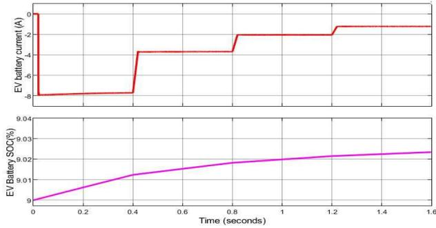
Fig. 6. EV battery charging current and % SOC.
