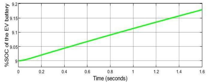
Fig. 13. Charging of EV battery represented by increasing %SOC
