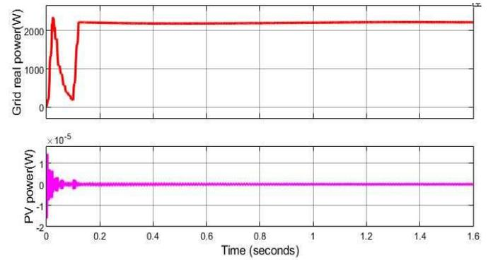
Fig. 11. Grid supplied power when PV output power is zero
