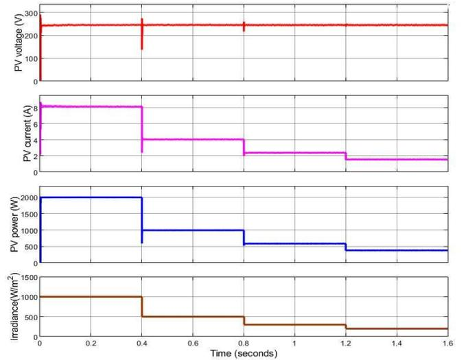
Fig. 5. PV Voltage, current, and power with a variation of irradiance.
