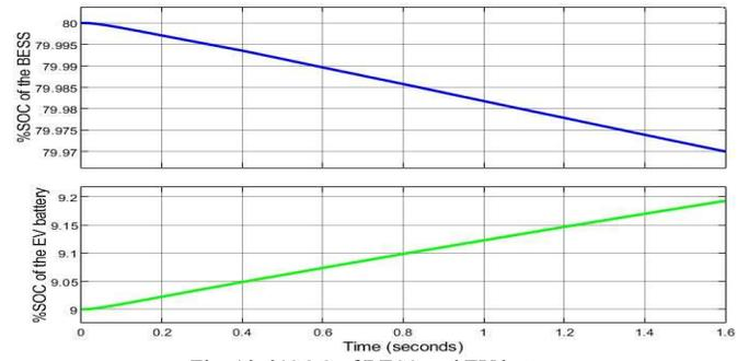
Fig. 10. %SOC of BESS and EV battery
