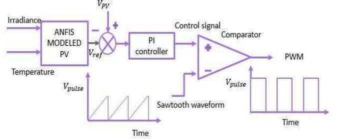
Fig. 3. ANFIS voltage-controlled MPPT
