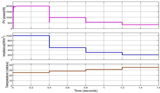
Fig. 8. Output power, Irradiance, and temperature of PV array.
