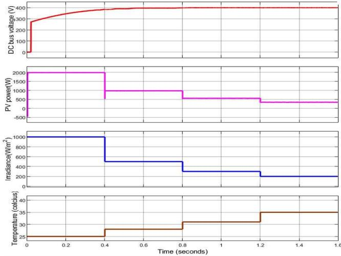
Fig. 9. DC bus voltage, PV output power, Irradiance, and temperature of PV array.
