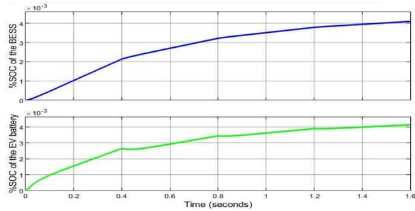
Fig. 7. % SOC of BESS and EV battery
