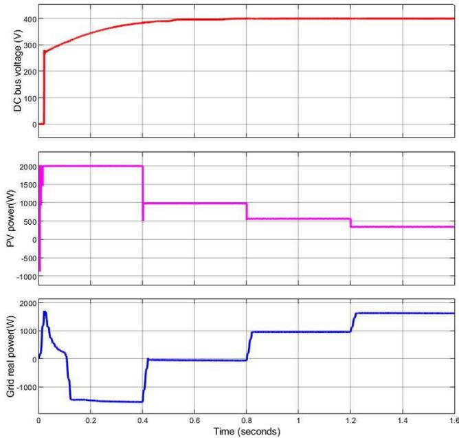
Fig. 14. DC bus voltage, Power supplied by PV array, and Grid real power
