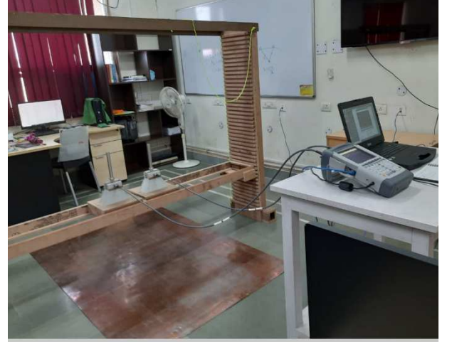
Fig. 3. Laboratory Setup of bi-static air-PEC scenario in GPR lab at NIT Rourkela
