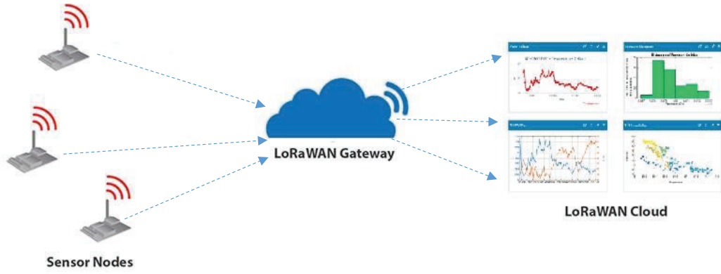
Fig. 2: The architecture of LoRaWAN with sensor node and gateway as in a practical application.
