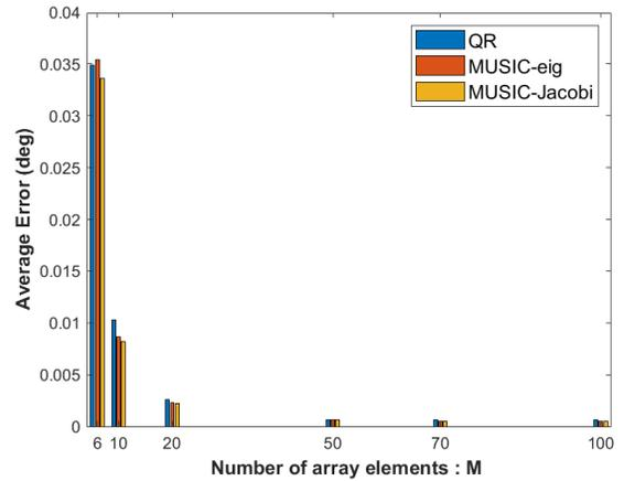
Fig. 4. Average error versus number of array elements  $M$
